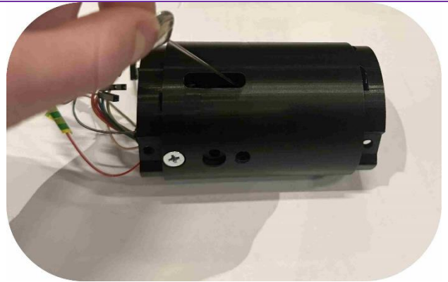
Figure 18 – master switch access photo
