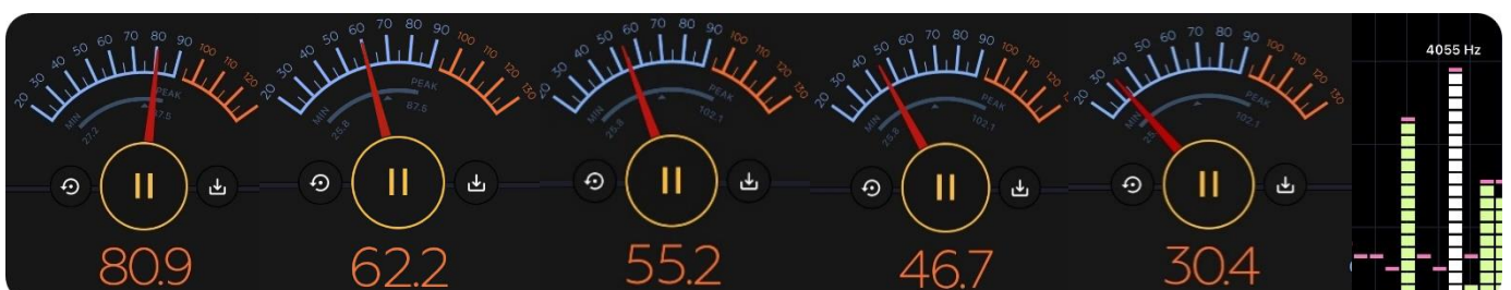
Figure 29 – Buzzer Loudness Values (from left) at 1m, 10m, 20m, 50m, and 100m from the Source, Frequency
